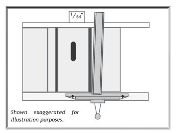
Figure 14. Lead adjustment.
